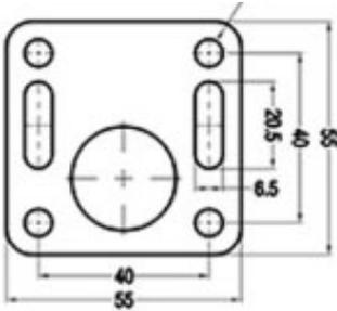
The installation measurements for the base of the ball can be seen here. Screw hole diameter is 6.5 mm and distance between the holes 40 mm.
